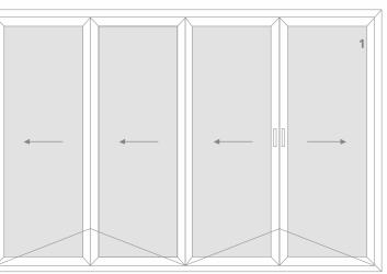
**DESIGN FORMAT SLIDE AND FOLD**  FRAME DEPTH **70MM**
